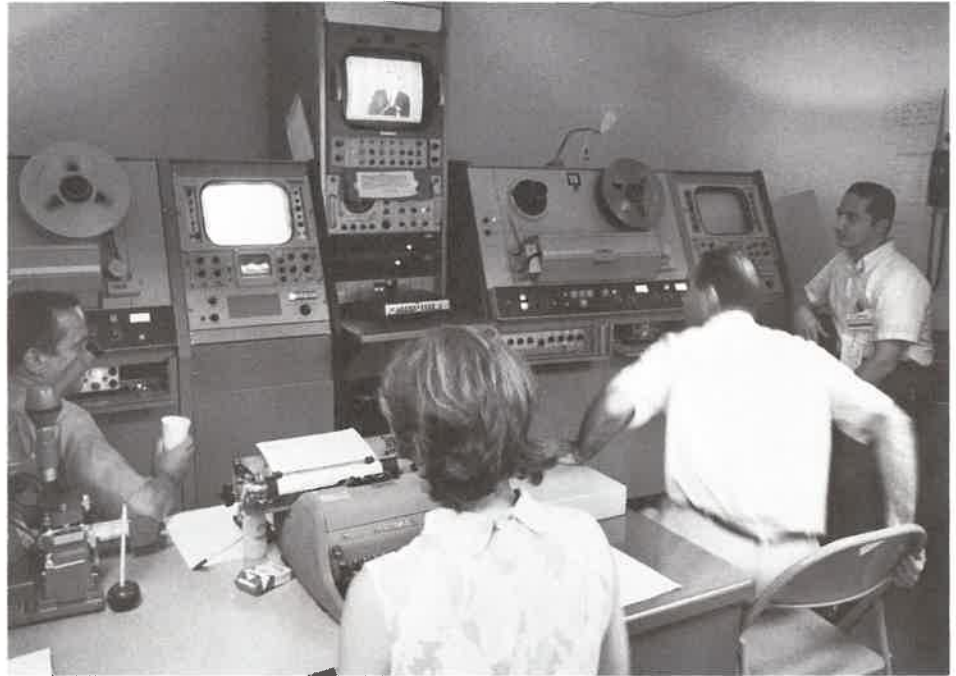
One of three dual VR-2000 equipped recorder stations set up by ABC in Chicago. Girl in foreground is logging a tape during recording to provide a fast access index and archival record. One station had an Ampex HS-100 Slo-Mo recorder for stills and slow motion.
